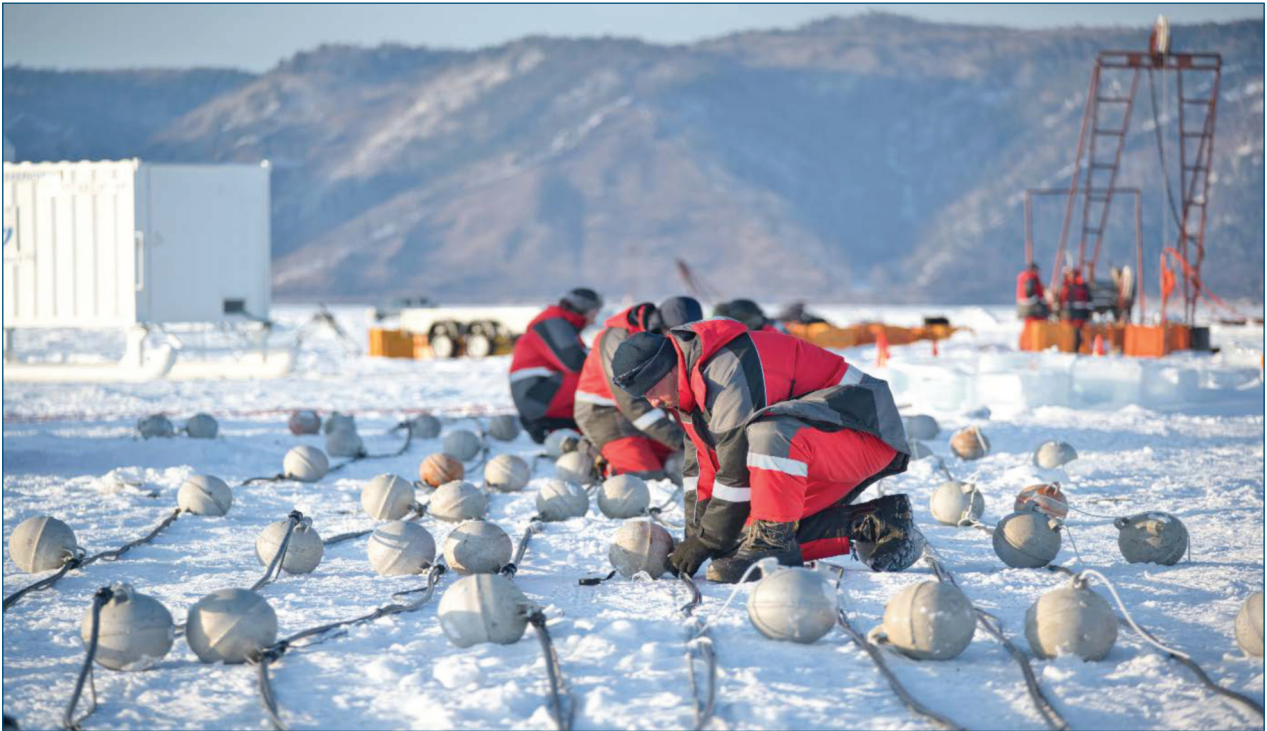
Fig. 12. Assembling the Baikal-GVD installation cluster garland
