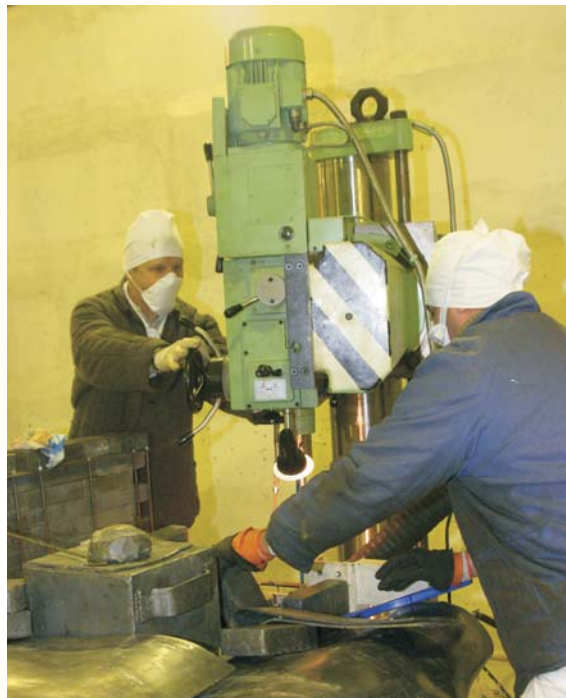
Frank Laboratory of Neutron Physics, 14 December. The IBR-30 reactor zone unloading: extraction of the fuel tanks (left), boring inserts out of the disc of the main movable zone (right)
