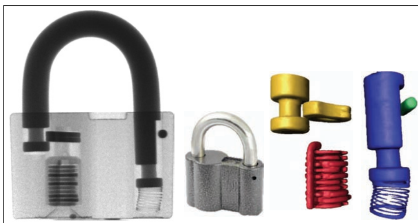
Fig. 2. Left: Neutron image and conventional photo of a padlock. Steel components of the lock (spring, locking mechanism, shackle) are clearly visible against its aluminium body. Right: Three-dimensional model of the internal mechanism of the padlock reconstructed using neutron tomography data. The individual components of the lock are displayed in different colours
