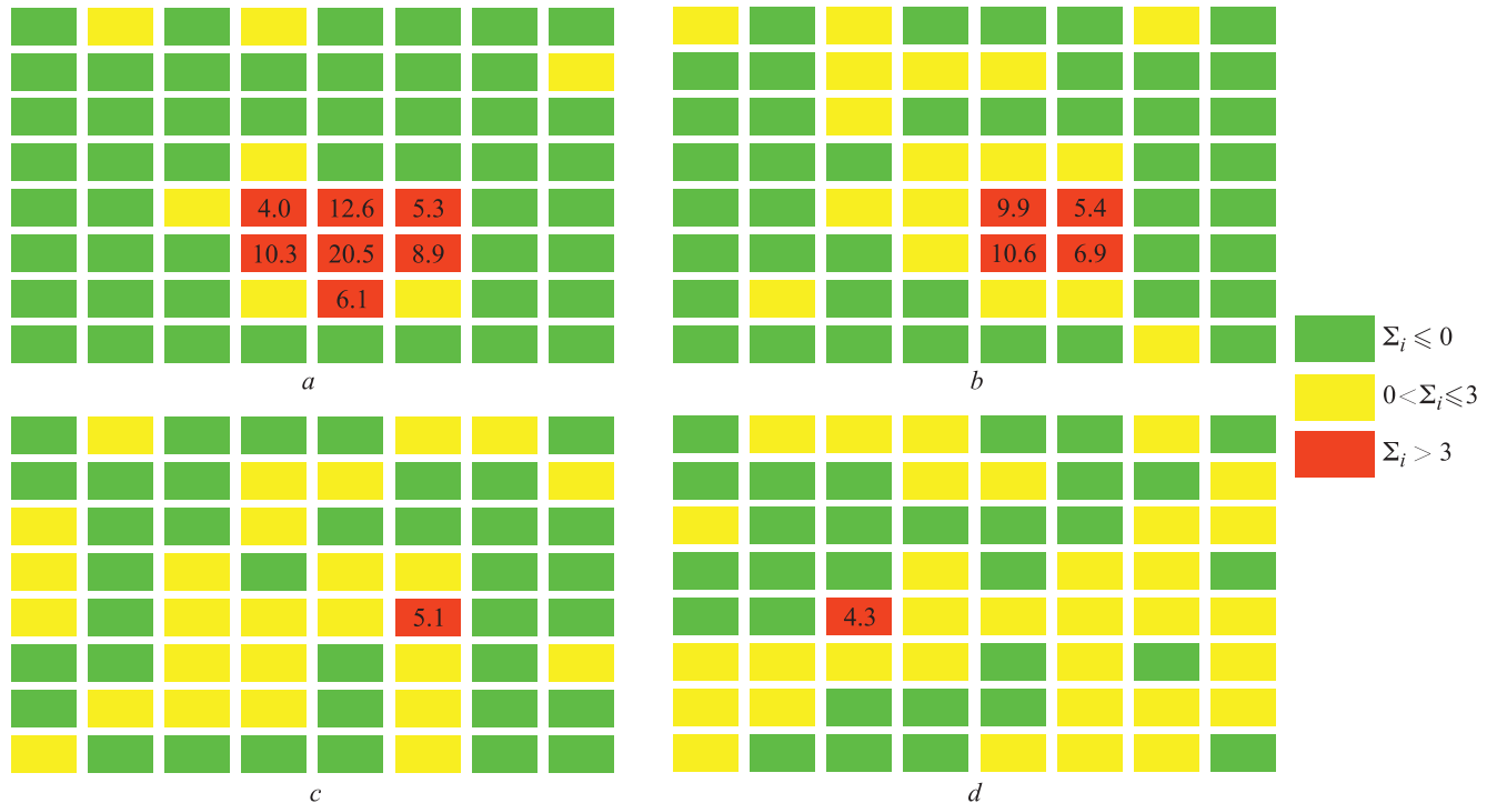
Fig. 1. Distributions \Sigma_i = (N - N_i)/\sigma for irradiated kimberlite samples with diamond simulants of different mass inside. The masses and diameters of the simulants were 11.2 g and 20 mm (a), 5.2 g and 15 mm (b), 1.78 g and 10 mm (c), and 1.15 g and 8 mm (d). Yellow cells are with 0 < \Sigma_i \leq 3 ; green cells are with negative \Sigma_i ; red cells are with \Sigma_i > 3 (numerical values of \Sigma_i are given inside)
