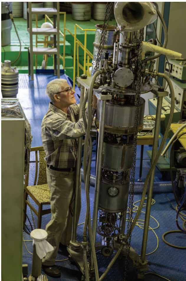
The Frank Laboratory of Neutron Physics, June. The cryostat of the KOLHIDA set-up. The assembling of sensors for measuring ultralow temperatures
