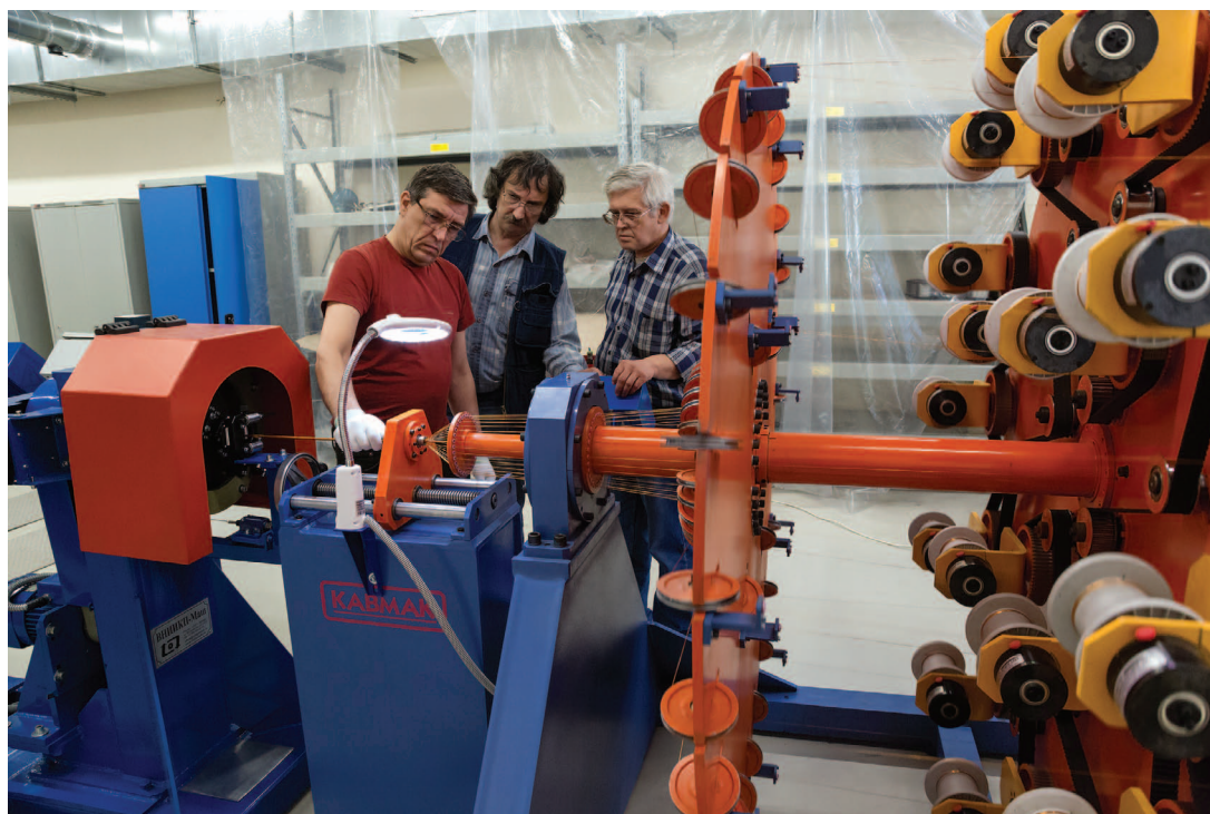
The Veksler and Baldin Laboratory of High Energy Physics, May. A production line of the tube superconducting cable
