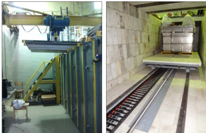
Fig. 2. General view of passive shielding: from the outside and inside. The range of detector dislocation is 6–12 m from the reactor core center
