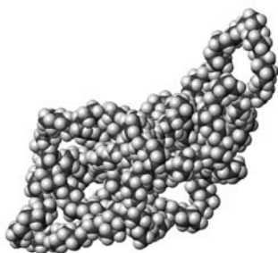
Fig. 1. Initial configuration of a polyethylene chain (black circles — carbon atoms, white circles — hydrogen atoms)
