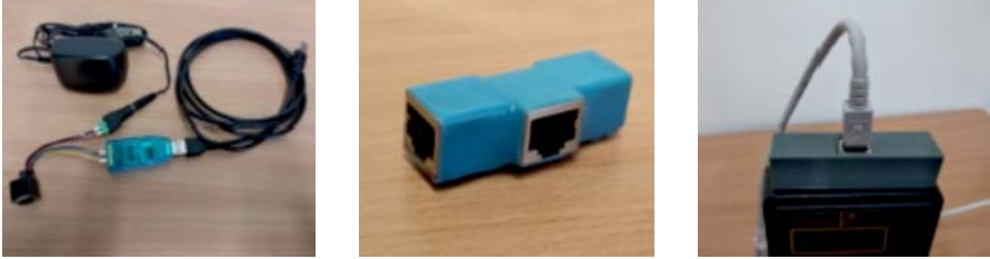
Fig. 8. The part of the dosimetry system. Left: the way of connecting power supply and RS-485 bus signals from USB-RS485 converter; center: T-branching signals on the RS-485 bus; right: new EKO-C connector
