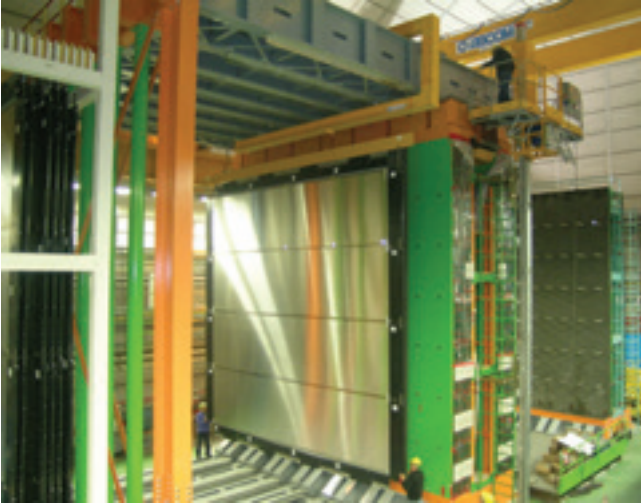
Insertion of the first Target Tracker wall in OPERA detector in 2004. Each wall has a dimension of 8 \times 8 \text{ m}^2
