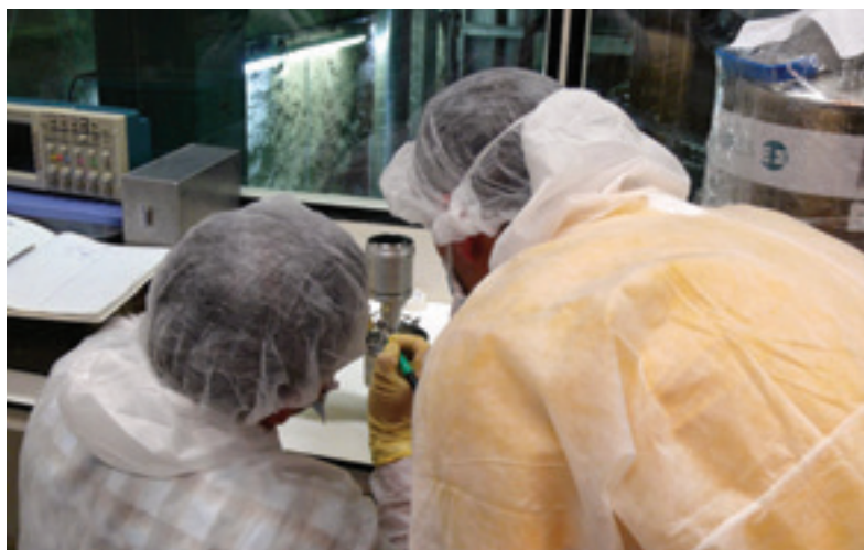
Members of JINR EDELWEISS group E. Yakushev and S. Rozov perform installation of 241 g point contact detector into a cryostat. Photo taken in June 2011, EDELWEISS clean room in the LSM laboratory
