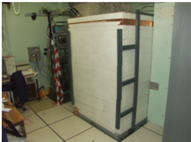
TGV-2 spectrometer mounted at the Modane underground laboratory
