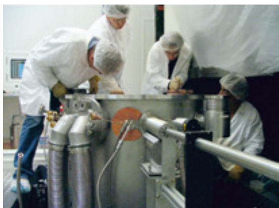
Few pictures representing the EDELWEISS cryostat assembly and detectors installation and wiring
