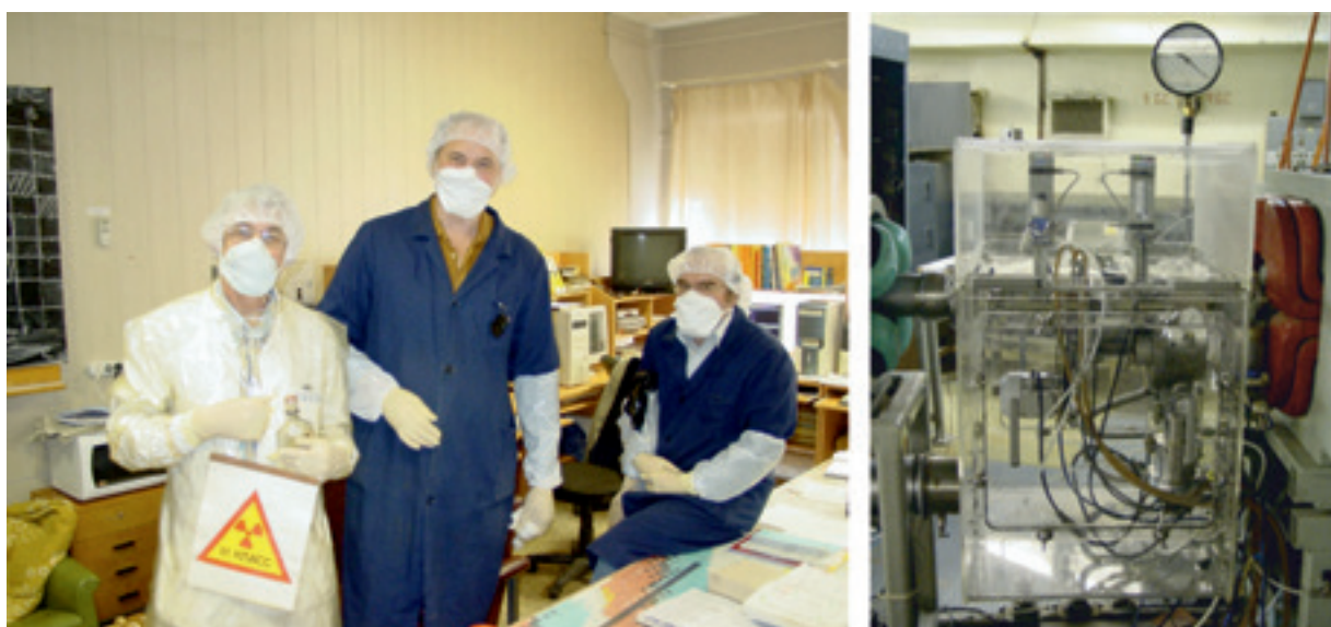
Left: Physicists prepare to install the ^{210}\text{Pb} radioactive-target chamber. Right: Target containment chamber in place
