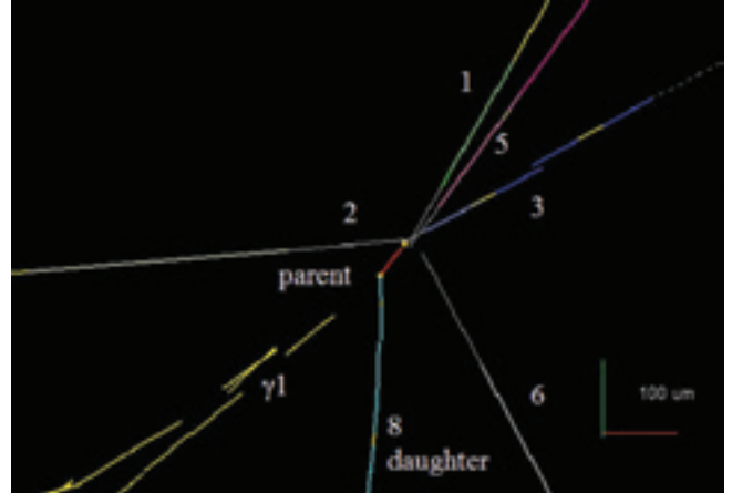
First OPERA \nu_\tau candidate discovered in 2010. This event could come from the decay of the tau lepton into hadrons produced by a tau neutrino interaction
