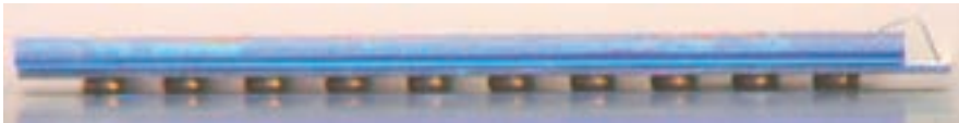
Side view of a Medipix3 silicon detector assembly connected to a printed circuit board using a ball grid array. TSV's are used to connect the ball grid array to the front side of the ASIC.
