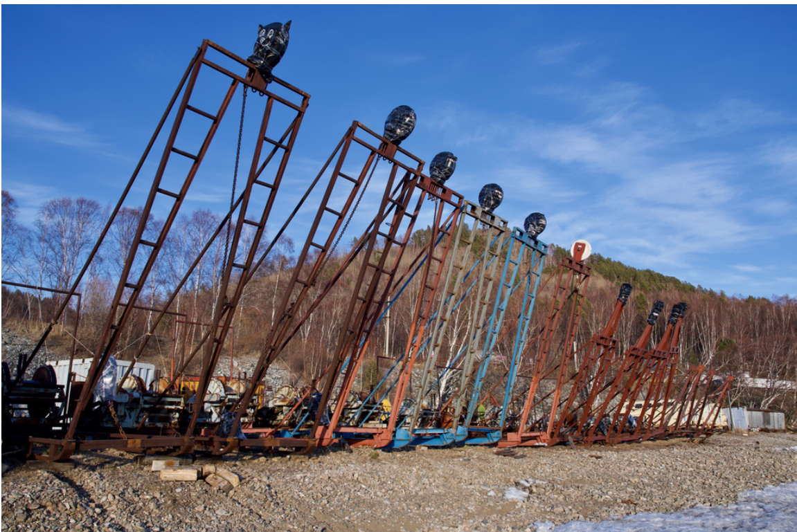
Windlass is the main device for carrying out deep underwater assembly on ice
