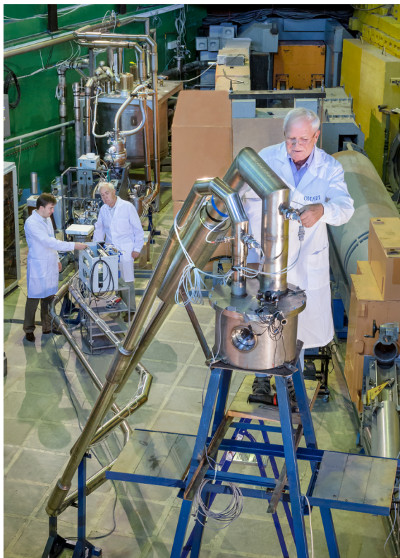
A test bench of the cryogenic neutron moderator of IBR-2
