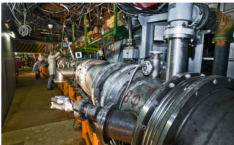
The Nuclotron – a superconducting accelerator of relativistic nuclei and heavy ions
