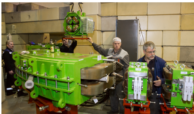
Superconducting magnetic system for the ECR source
