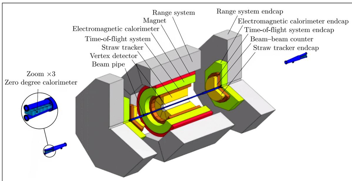
Fig. 6. Upgraded configuration of the SPD detector
