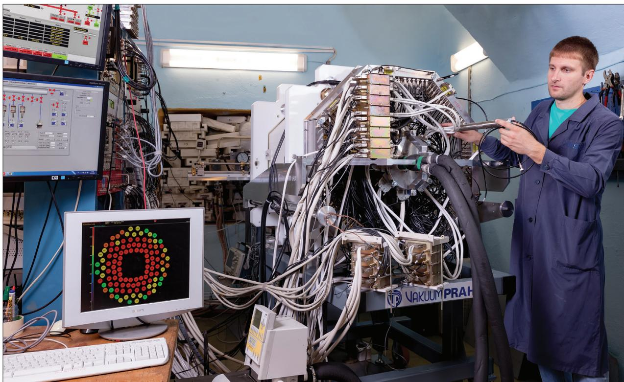
The Flerov Laboratory of Nuclear Reactions. The SFiNX detector system of the SHELS separator for studies of the properties of the spontaneously splitting short-lived nuclei obtained in reactions with heavy ions
