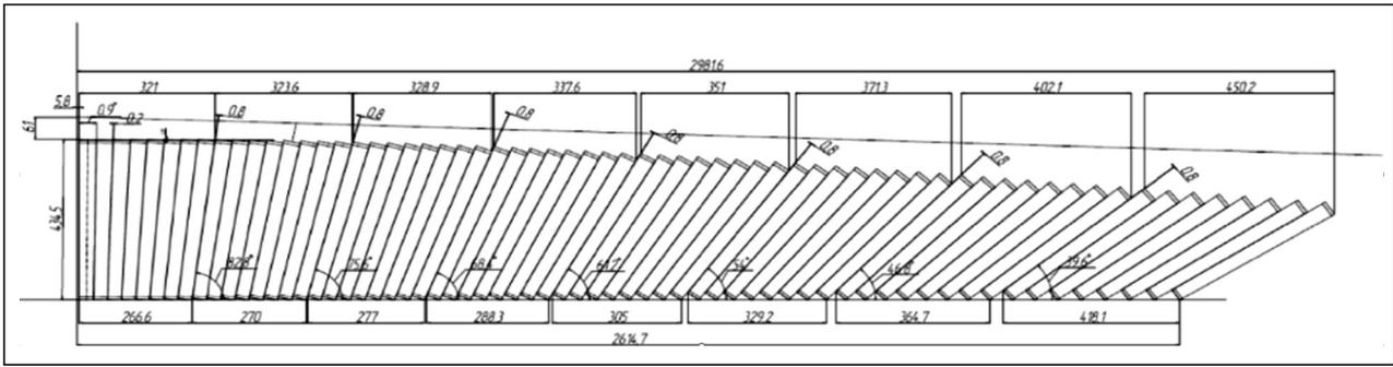
Fig. 3. Layout of the towers in the half-sector of the electromagnetic calorimeter with a projective geometry
