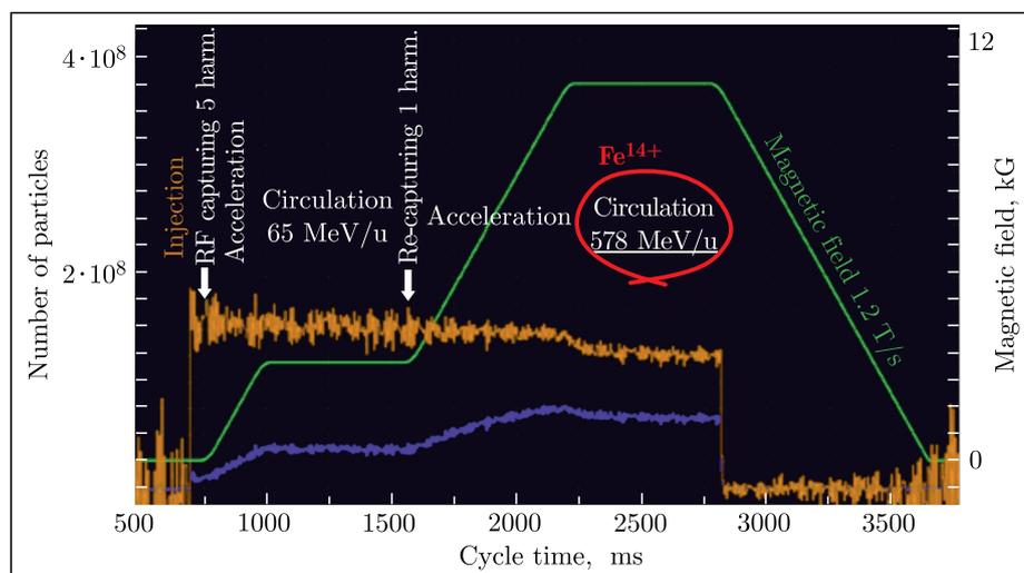
Fig. 1. A signal from the beam current sensor in the Booster
