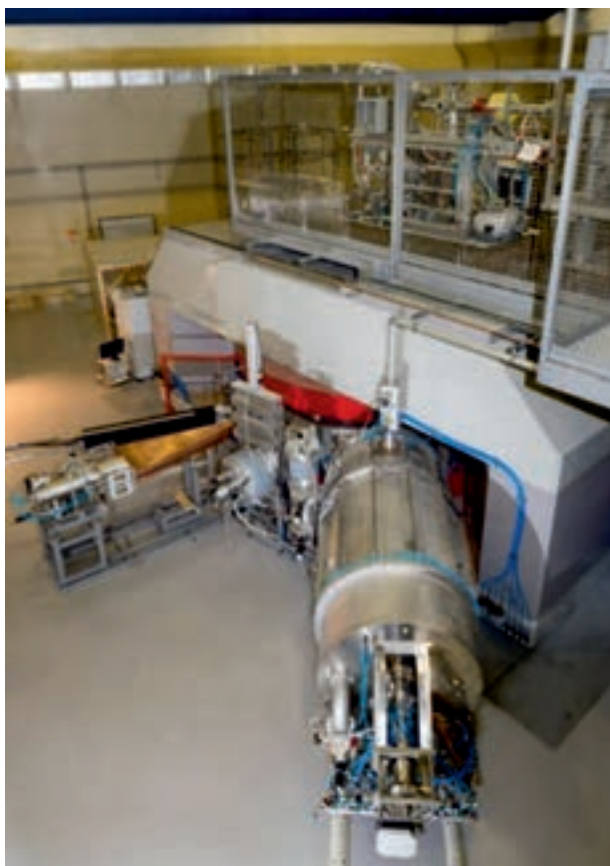
Basic element of the SHE Factory, the DC-280 cyclotron
