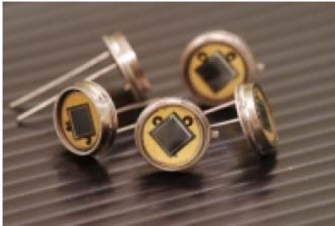
The silicon-based multipixel avalanche photo diodes (left) and MAPD test facility at Charles University (right)
