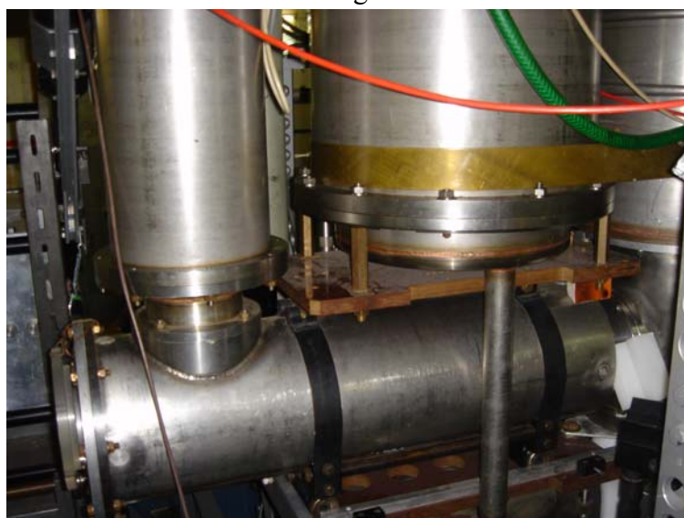
Superconducting magnet system (jointly created by JINR and Czech specialists) for the Frozen Polarized Target at Van de Graaff accelerator of Charles University (Prague)
