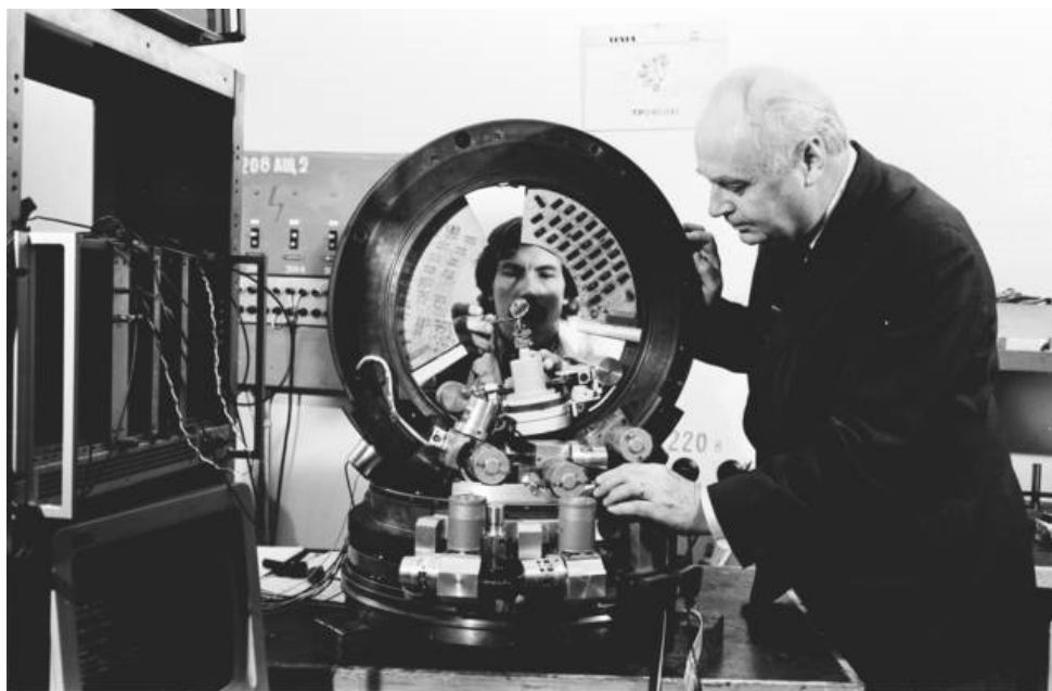
Prof. C.Šimáně (right) and his co-worker check very accurate goniometry device which was used for adjustment of target mono-crystals in the neutron beam of IBR-2 (1981)
