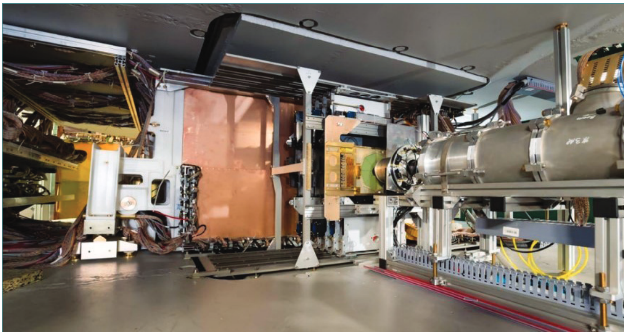
Trigger detectors of the target area and the central tracking system inside the BM@N spectrometric magnet
