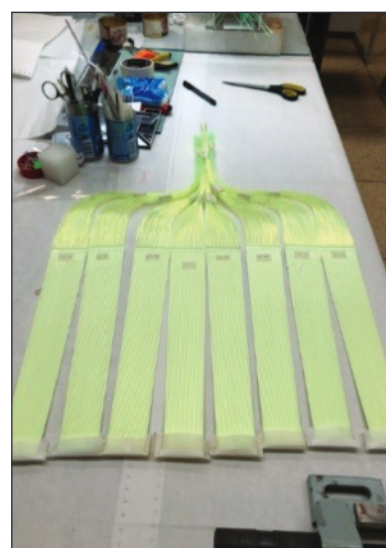
Left: ASTRA-M detector at the FSD spectrometer. Right: External view of individual elements of the ASTRA-M detector. The element is a (Ag)/ 6 LiF scintillator plate, which is shaped like a time-focusing surface with glued wavelength-shifting fibers that transmit the light flux from the neutron capture site to the photomultiplier
