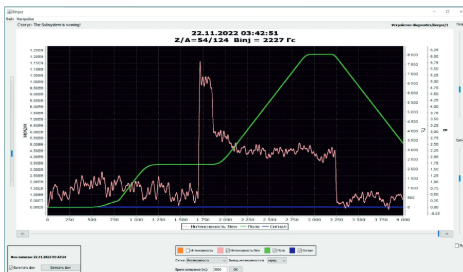
Cycle of the Nuclotron magnetic field and the intensity of the beam of xenon nuclei, measured by a parametric current transformer, during setup tuning for the BM@N experiment. The intensity of the accelerated beam is approximately 10^7 particles
