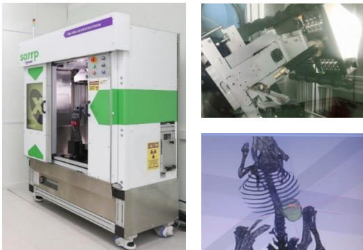
Laboratory of Radiation Biology SARRP facility for modeling conformal radiation therapy on laboratory animals
