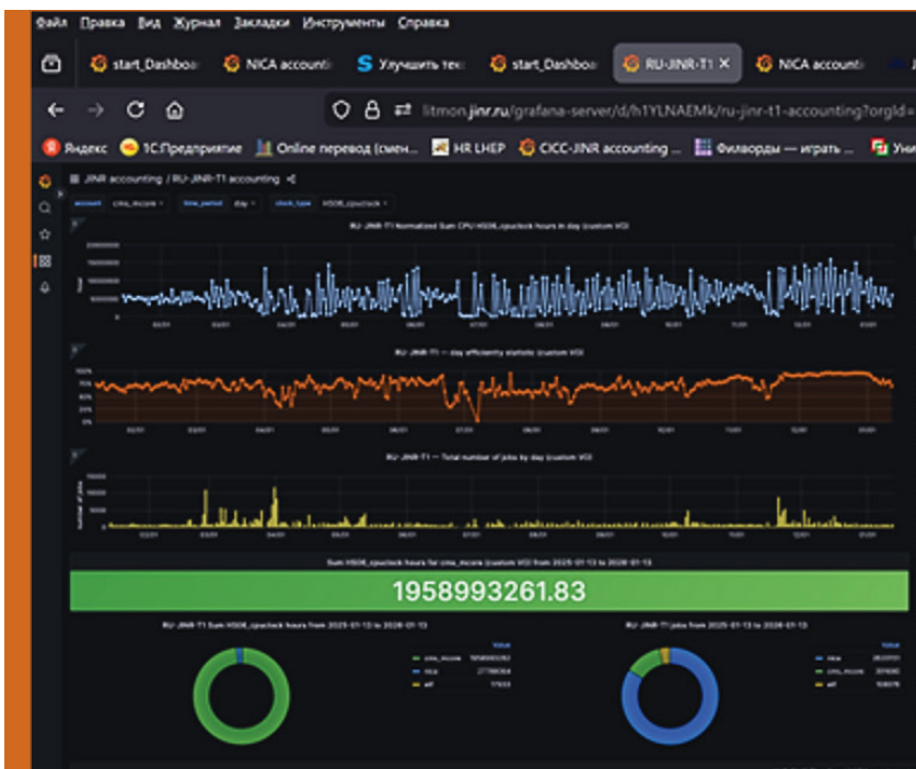
Fig. 8. General information screen of the Tier1 CMS grid site task accounting system
