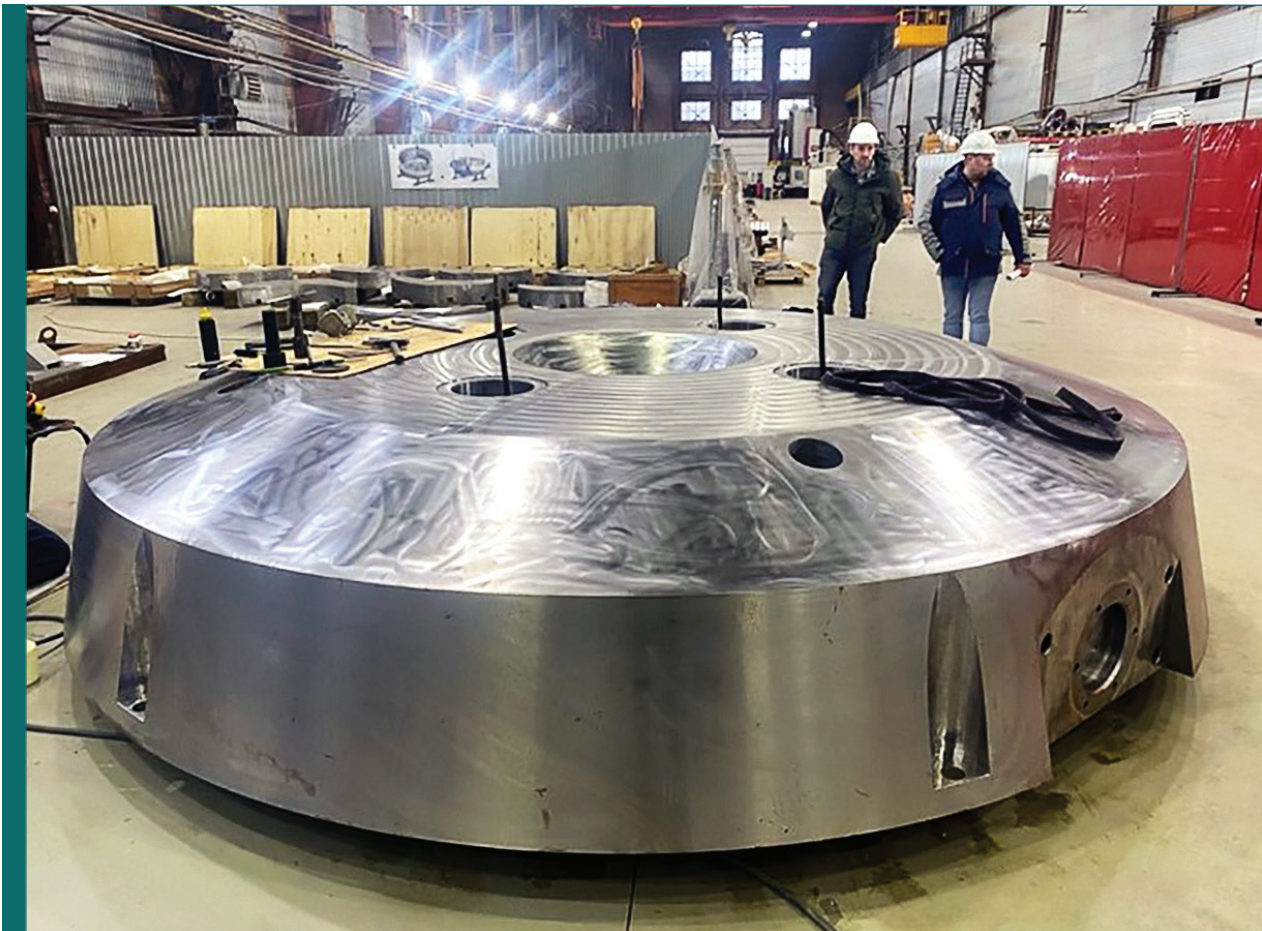
The medical superconducting cyclotron MSC-230 is under construction. The cyclotron yoke with a yoke-top lifting system
