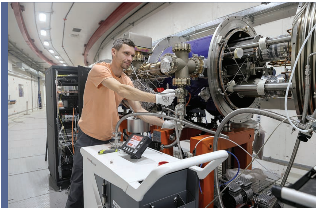
Checking the tightness of the Collider beam chamber
