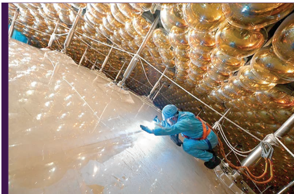
Jiangmen (China). A worker inspects the material of the acrylic sphere of the JUNO central detector
